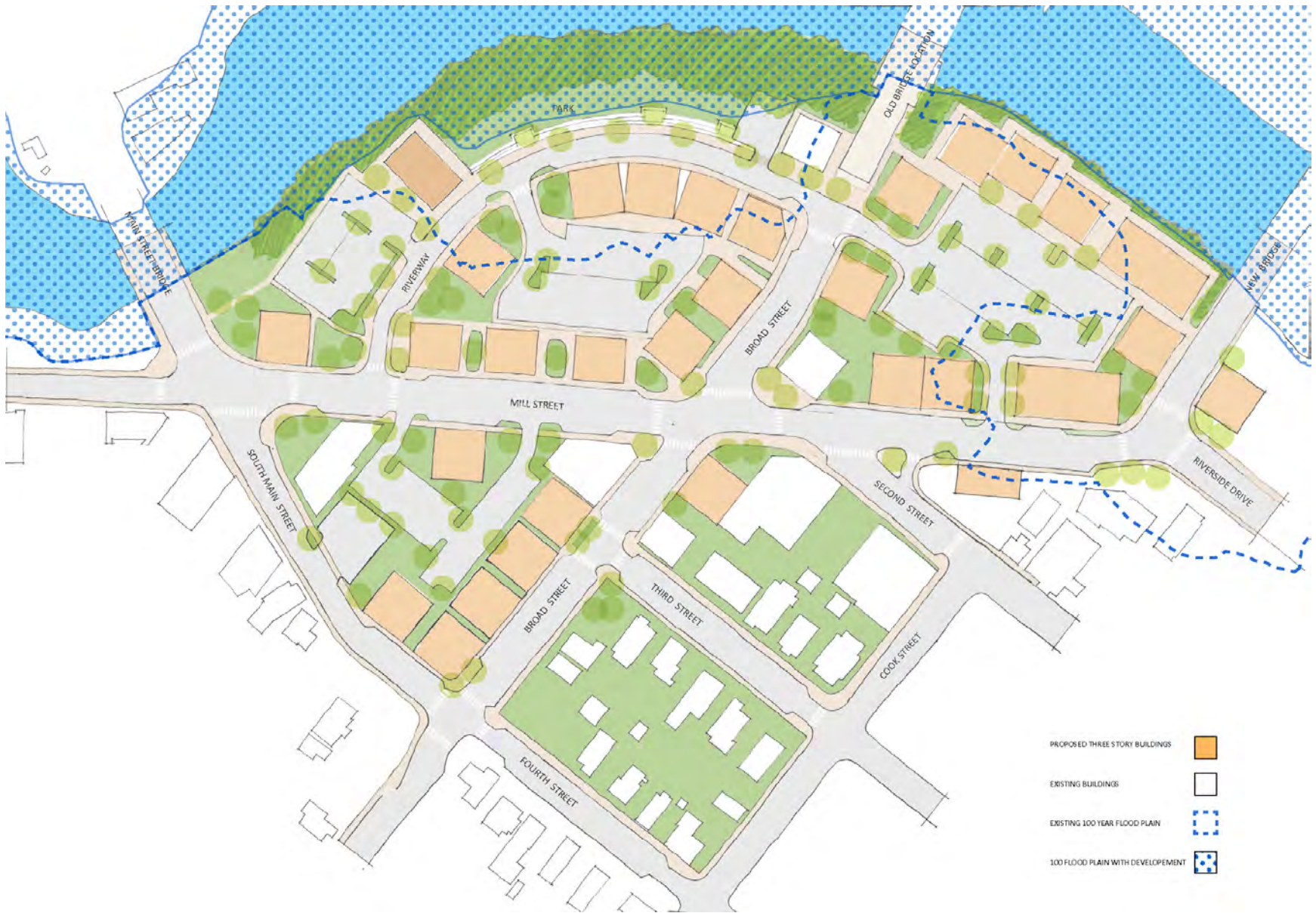
Figure 62: Extent of 100-Year Flood Plain After Relocating Lown Peace Bridge and Creating the Riverway
