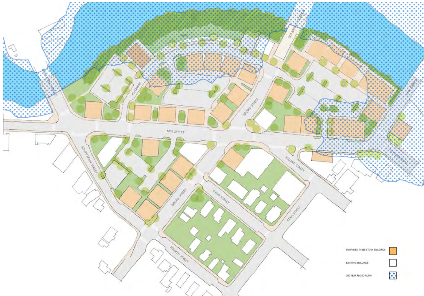
Figure 61: 2014 New Auburn Village Center Master Plan with Extent of Existing 100-Year Flood Plain – Elevation 135'
